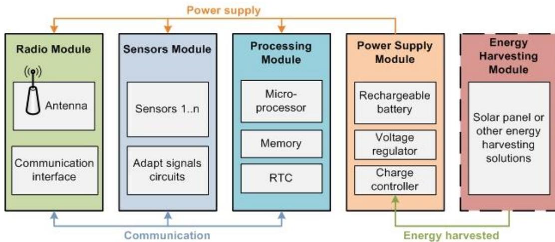
Fig. 2. Network device (node) architecture
