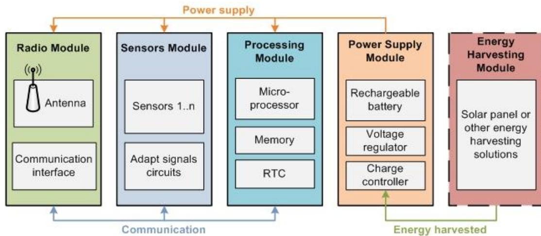
Fig. 2. Network device (node) architecture
